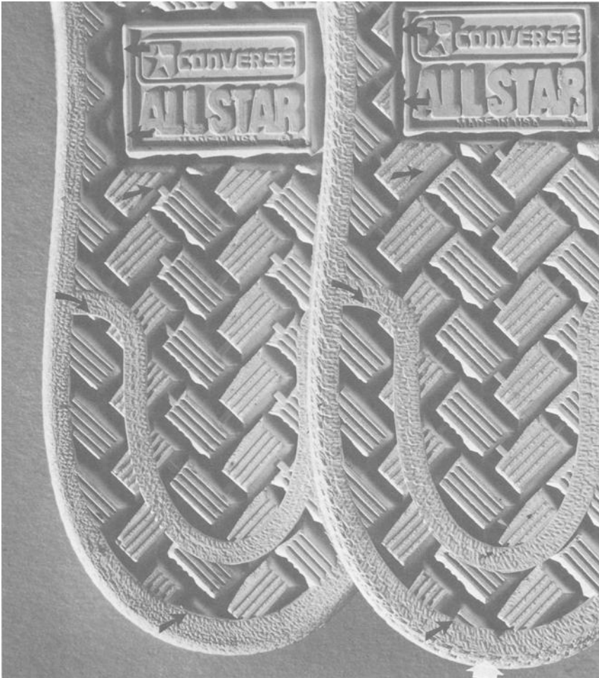
FIG. 11—Respective portions of outsoles from two different molds, same size and design, made by the same mold manufacturer at the same time. Note the variations in the gross design. Also note the hand stippling on the border (white arrow).
