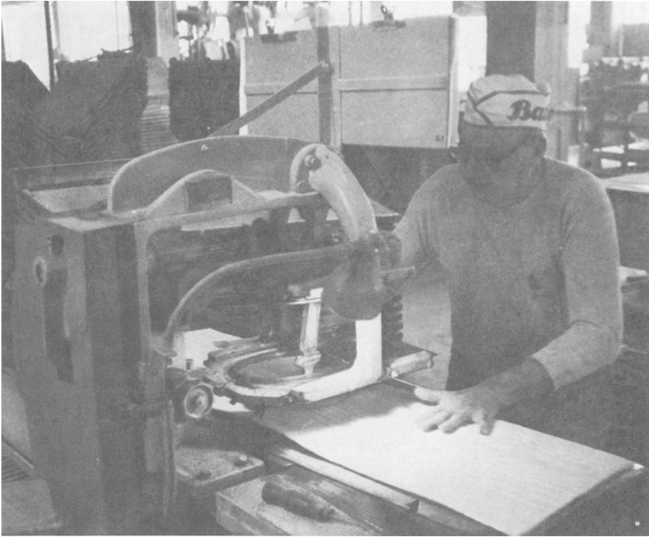
FIG. 8—A “slab” of calendered outsole material is manually fed beneath the cutting head of the Wellman Outsole Cutting machine.
