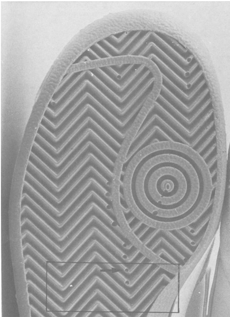
FIG. 19—Polyurethane direct injected outsole. Note how the air bubbles favor the valleys of the design.
